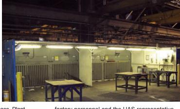
At Wyman-Gordon's Grafton, Mass. Plant, workers hand grind metal to remove defects from the forging process and excess flash. Parts range from 2-ft. to 10-ft. wide, up to 22-ft. long, and can weigh under 100-lbs., or over 15,000-lbs.
