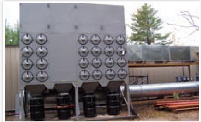
CLARCOR Industrial Air custom designed an extended dirty air plenum to collect particles in all shapes and sizes.
