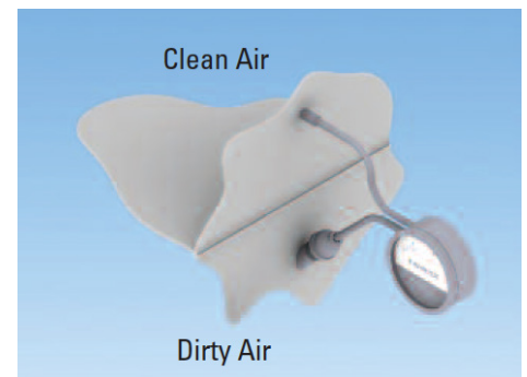
This cutaway image shows the correct installation of an automatic clean-on-demand system's differential pressure gauge.
