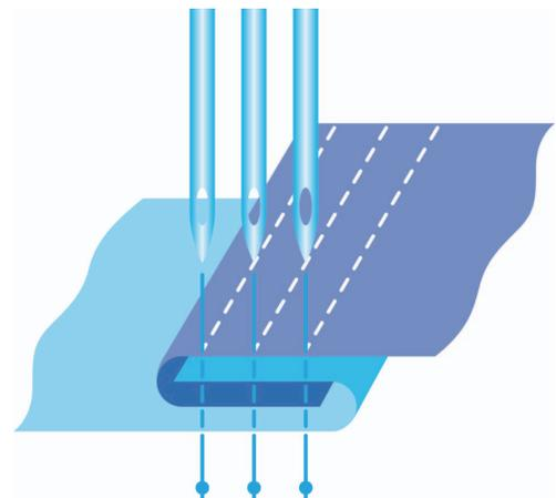
Figure 2. Stitching construction.
