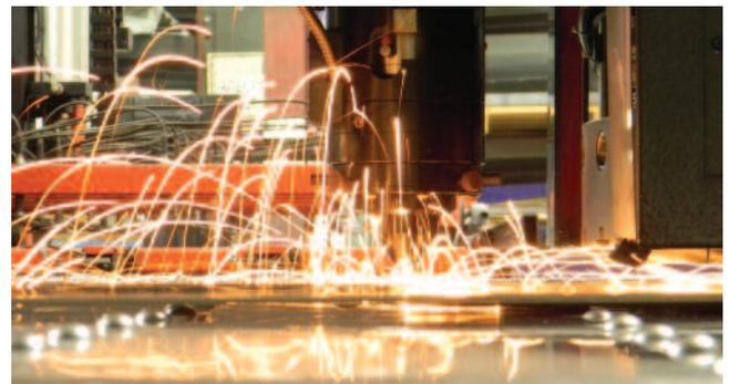
Fume is generated at the point of cut, as well as by the molten metal slag resulting from the cut. In some cases, a three- to six-inch water basin sits directly below the cutting process to capture and immediately quench the molten material and reduce the generated smoke and resulting fume.
