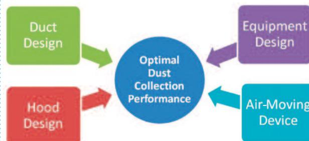
considerations must be made in order to design a proper dust collection system that achieves optimal performance.
