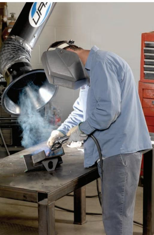
Fig. 1 — Capturing the fume at the source, as shown here, yields the best results and requires the least amount of energy.
