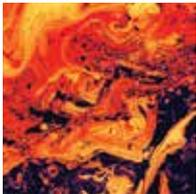
In order for sodium sulfate to attack turbine materials, it must be in a molten state. However, the melting point of  $\text{Na}_2\text{SO}_4$  shifts downwards when in the presence of sodium chloride. This reduction can be from over 1600°F (~875 °C) to as low as 1110°F (~600 °C), which greatly increases the potential for corrosion.
